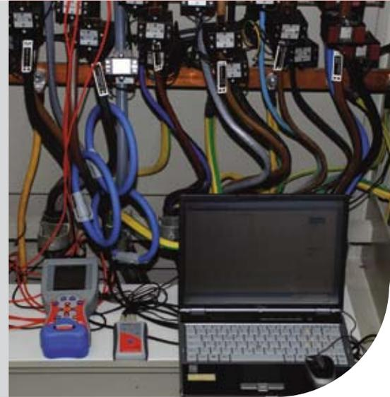
**PowerQ** is a lightweight, handheld, 3-phase analyser for quick power quality assessment in low and middle voltage systems.
