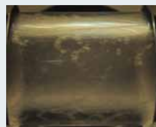
80% dryness fraction ( x = 0.8 ) 20% condensate (with annular flow)
