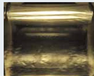
90% dryness fraction ( x = 0.9 ) 10% condensate (with wavy flow)
